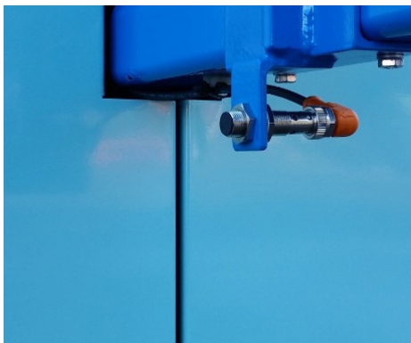
The position of the limit switch can be adjusted.
