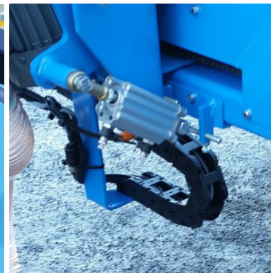
Adjust scraping cylinder speed on the one-way flow control valves.
