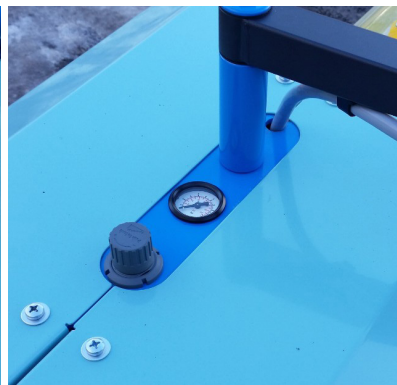
Pressure regulator and pressure gauge for adjusting the scraping pressure.
