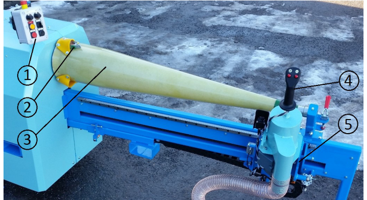
On the picture you see; control panel(1), clamp(2), beam (3), joystick (4), wagon(5), the wagon is in home position.
