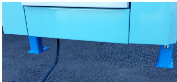
Connect the machine to 1-phase wall-socket (16A) and compressed air.
