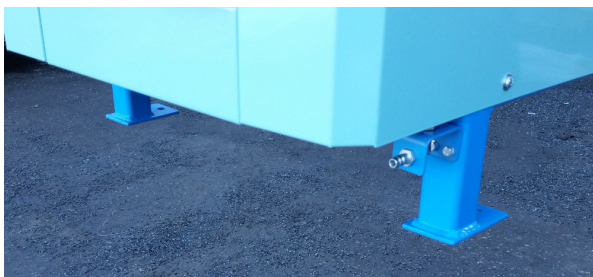
Bolt the machine to the floor with 3 pcs M10x100mm anchor bolt.
