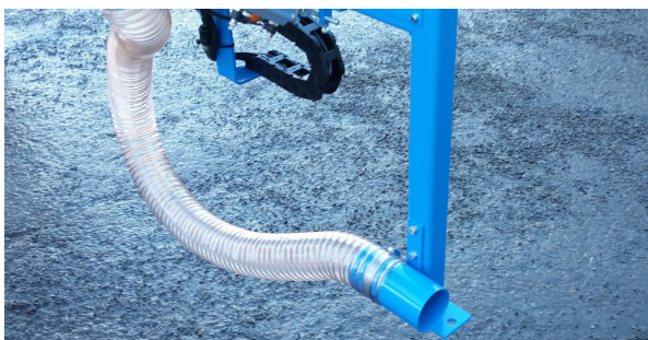
Connect hoses from the ?properties? fat suction system to the machine.
