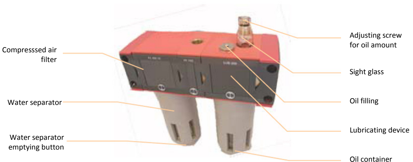
Fig. 2 Compressed air filter and lubricating device
