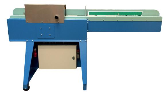
When the machine is started the chain with the skin transporter runs continuously. The skin is put on one of the hooks with the back side facing out. After that it gets pulled through the machine from left to right and then pushed out of the machine.
