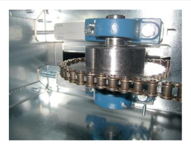
• The bolts by the bearing housing need to be loosened. Tightening takes place from outside using the tightening bolt.
