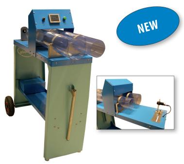
Jasopels has developed a length measuring device which will help you on your farm. The device is available with one or two censors which measure the mink with ultrasound.
