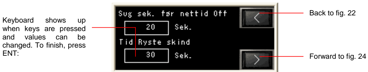
Fig. 23 Setting the startup of suction devices etc.
