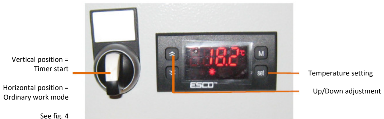
Fig. 3 Temperature settings & auto/manual mode settings
