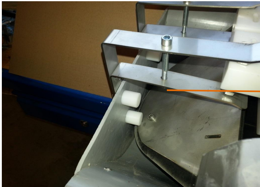
Fig. 6. Installation of a plastic stop.
