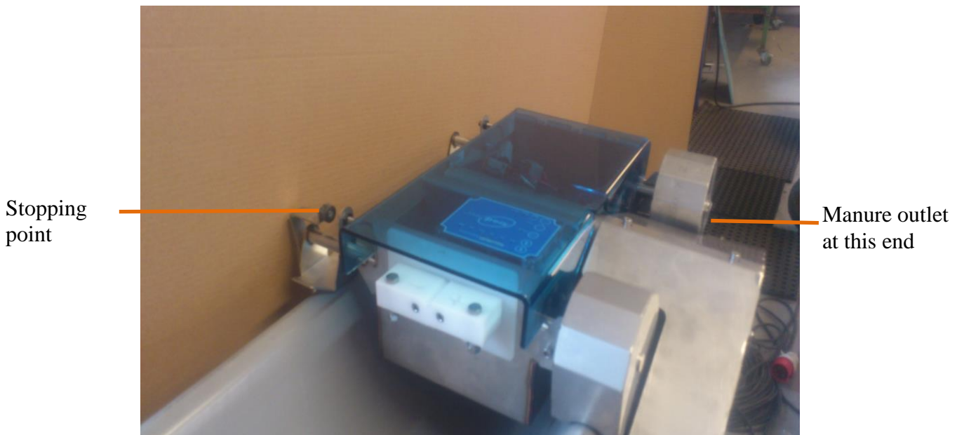
Fig. 9. Sensor at manure outlet at this end.
