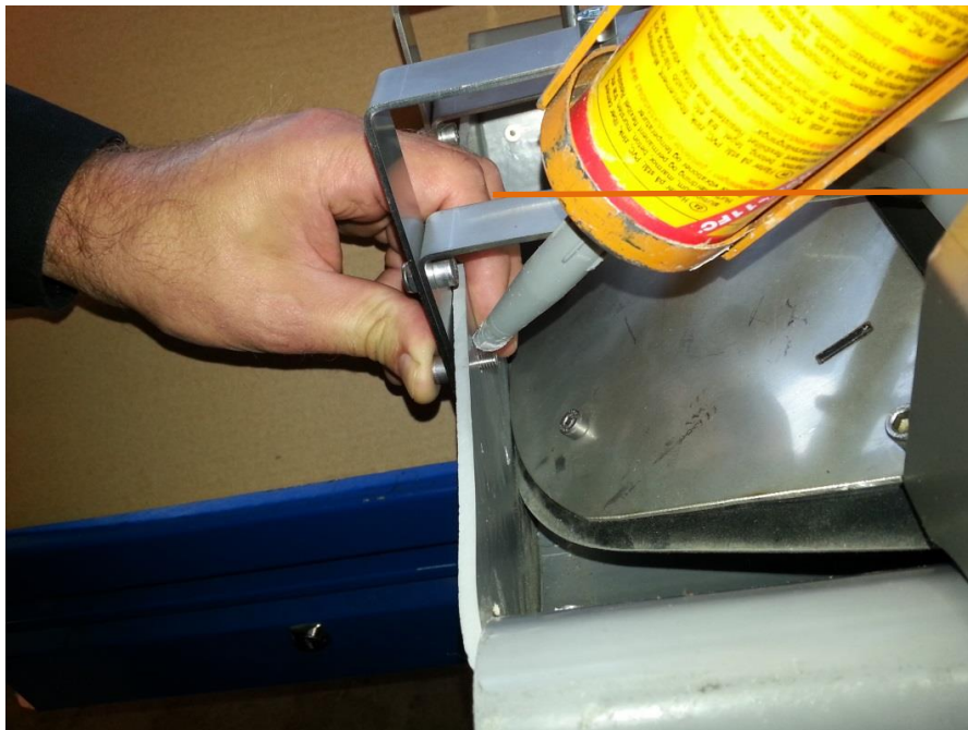
Fig. 5. Sealing the screws.
