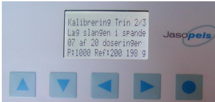
Figure 7 Calibrating of portioning unit, step 2
