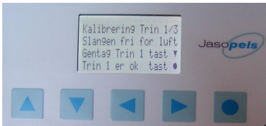
Figure 6 Calibrating of portioning unit, step 1
